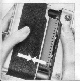
Fit the camera back to the body again (see illustration), lightly press together, then turn back and fold down the latch.
